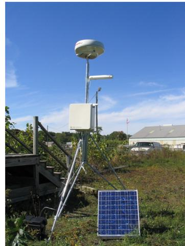
Fig. 1: OTG Prototype composed of solar panel, battery, data acquisition, wireless communications and marine radar.
