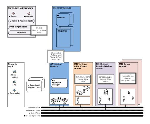
Figure 5-4. Cluster D utilizing ORCA control framework
