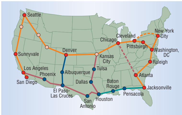
Figure 1. National LambdaRail. Using this backbone, the virtual testbed can support larger traffic volumes, with PlanetLab nodes aggregating traffic from local sites and feeding it to the backbone nodes.
