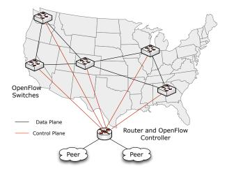
single controlling entity to determine the forwarding behavior of the underlying switches.
