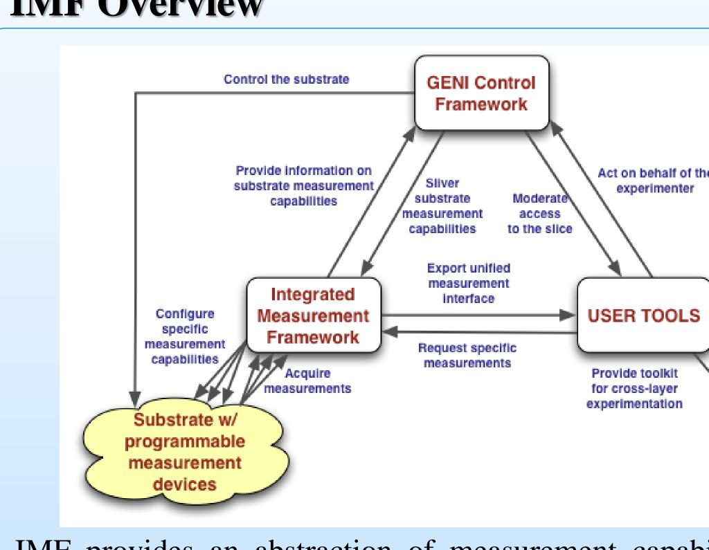
IMF provides an abstraction of measurement capabilities available within the GENI substrate by allowing experimenters to measure properties within the substrate, such as physical layer attributes (e.g. optical or RF power) and performance parameters (e.g. BER, packet loss, CPU usage) through a unified measurement interface.
