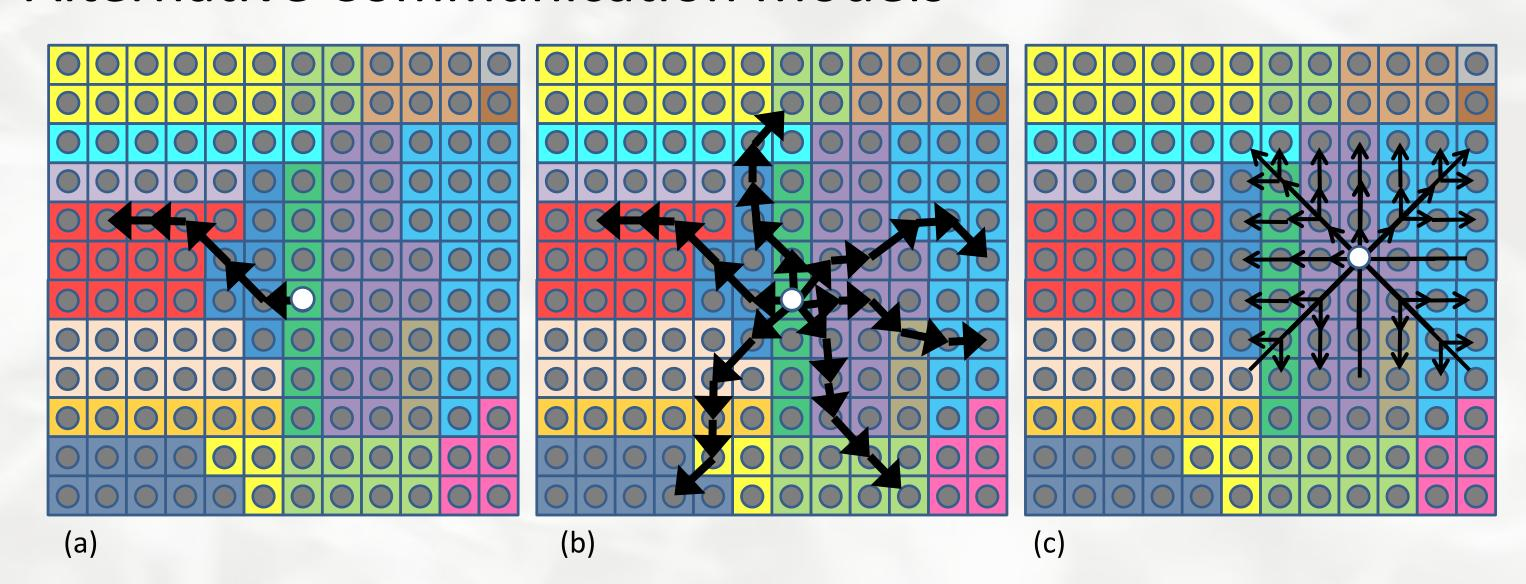
(a) *Basic model*: a single MSA leaves a trail from target in response to trigger. (b) *Alarm model*: multiple MSA are generated in response to trigger. (c) *Wasp model*: node Manager sends broadcast message to all neighbors in vicinity. Variations affect time to detect, resource use, and ability to detect non-local activity.
