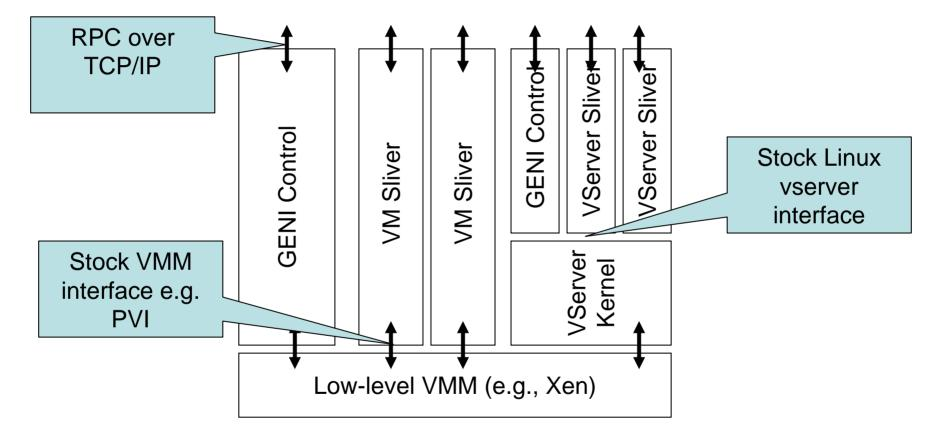
Experiments run as a vserver sliver or as a VM sliver Communicate with GENI management code (running as sliver) through RPC
