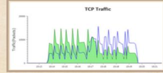
TCP Traffic Generate and analyze TCP flows. Iperf is used to create a flow and view the sawtooth behavior. Then, a second flow is introduced to show how TCP flows share a link.
