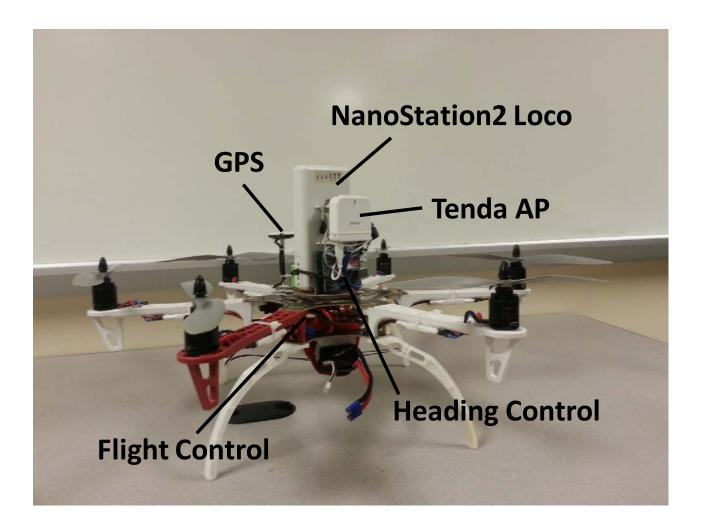
We use ARDUINO Atmega256 chip and LSM303 Ecompass sensor to guide the heading degree of the directional antenna. Also use XBEE to communicate with ground controller to indicate its height and get desired heading degree. The reading of the E-compass can offset the bias of the directional antenna so that the two antennas can face to each other precisely.
