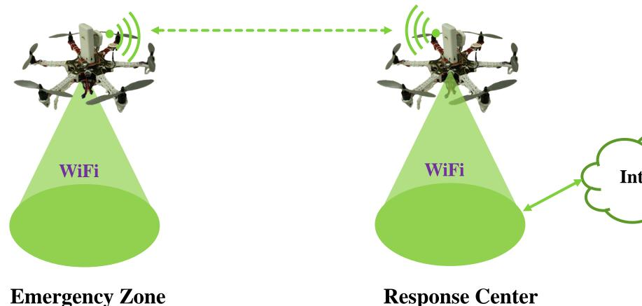
As shown in the above system for emergency scenario, the drone-carried WiFi system will provide fast-developed high flexible communication infrastructure to enable activities such as real-time video transmission, rescue team coordination, and phone/email communications.
