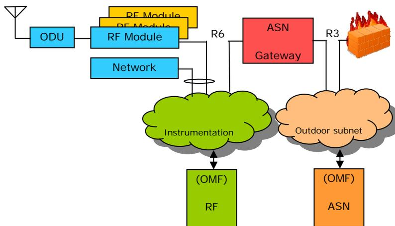
Fig 2: Integration of the WiMAX setup as a part of the ORBIT control and management framework.
