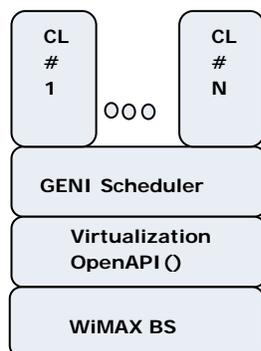
The GENI scheduler is responsible for controlling the access of the virtual machines (VMs) to the WiMAX BS and providing some SLAs to every slice. The GENI scheduler will work off the built-in WiMAX scheduler by exploiting its tight scheduling mechanisms to enforce slice fairness. It will create service flows, allocate and control access to each of them based on GENI defined slice policies. For the initial GENI scheduler design we are following a two pronged approach –
