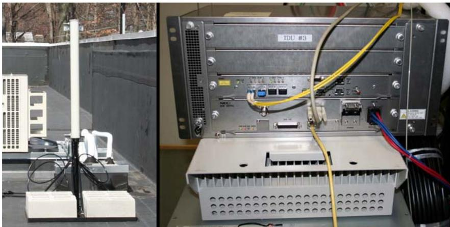
Fig 1: WiMAX antenna on the WINLAB Tech Center roof (elevation <6ft) and the base station with the power amplifier in the ORBIT control room
