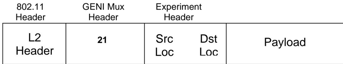
The GENI Mux header that denotes the sliver and virtual interface ids is included by an experiment specific client on the mobile and is assumed to be 21 for this example.
