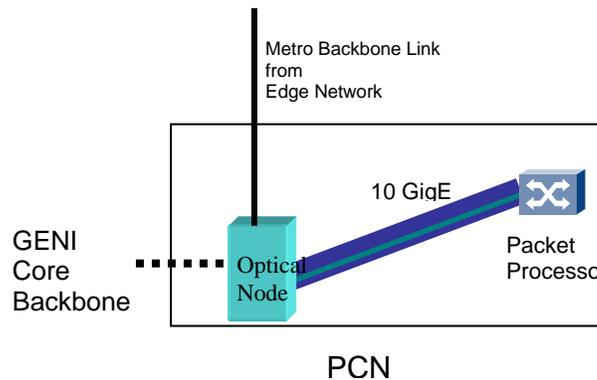
In this example, we assume that the PCN support cut-through routing at the optical domain for the traffic flow and, therefore, packets do not get out of the optical domain within the PCN. The packet traverses multiple PCNs and ultimately is sent to a destination GGW on Site B over a tail circuit.
