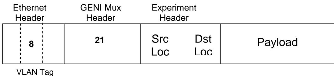
When the packet is received at the PAP, it is delivered to sliver/virtual interface 21. The sliver processes the packet and based on the experiment header, delivers the packet to the mobile located at the destination location.
