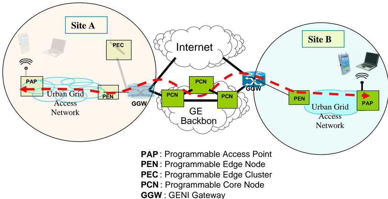
For an illustrative life-of-a-packet discussion, we consider an end-to-end experiment that requires the experimenter to receive a GENI slice with slivers running on the PAP and the PEN on site A and the PAP and PEN on site B but only requires a QoS guaranteed tunnel between the PAPs on site A and site B for bi-directional traffic flow between the PAPs (shown by the red
