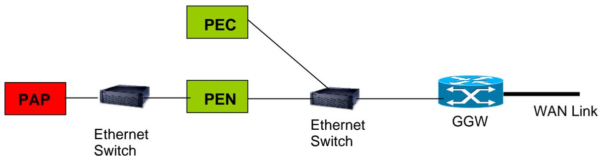
Traffic from the GGW at site B to the PAP would also be carried over two Ethernet hops with traffic differentiated using VLANs.
