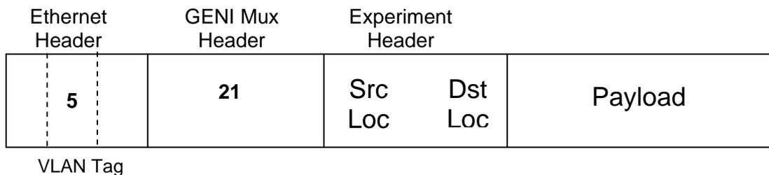
The PEN will strip the VLAN tag and look at the GENI Mux header to decide on the sliver to forward this packet. After processing, the packet will be forwarded to the PAP at site B with the appropriate VLAN encapsulation as shown.
