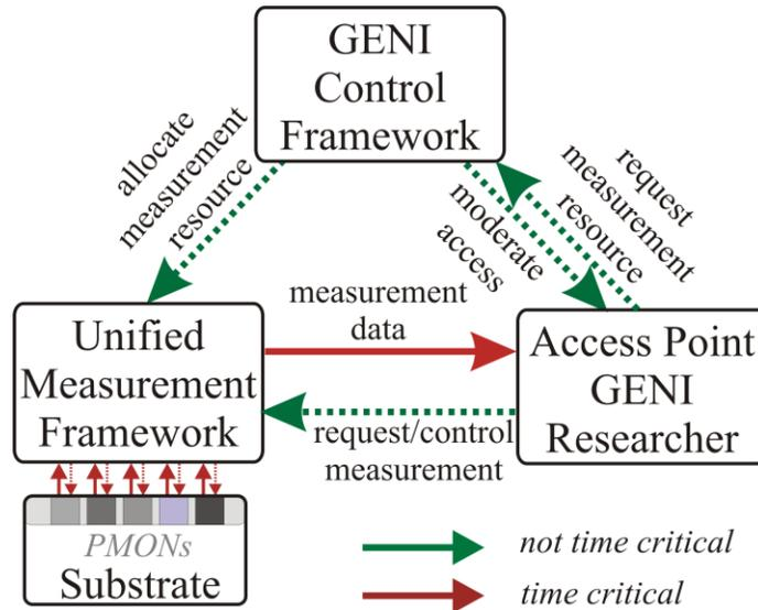
Figure 2-1: Schematic of interaction between performance monitors (PMONs) of substrate, unified measurement framework (UMF), control plane, and GENI researcher.
