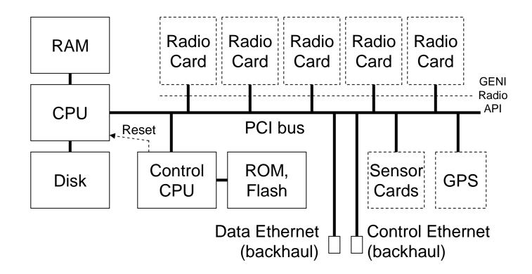
Goals: a) Run standard GENI component software without modification; b) Provide many radio upgrade paths; c) Use as core for Cognitive Radio kit
